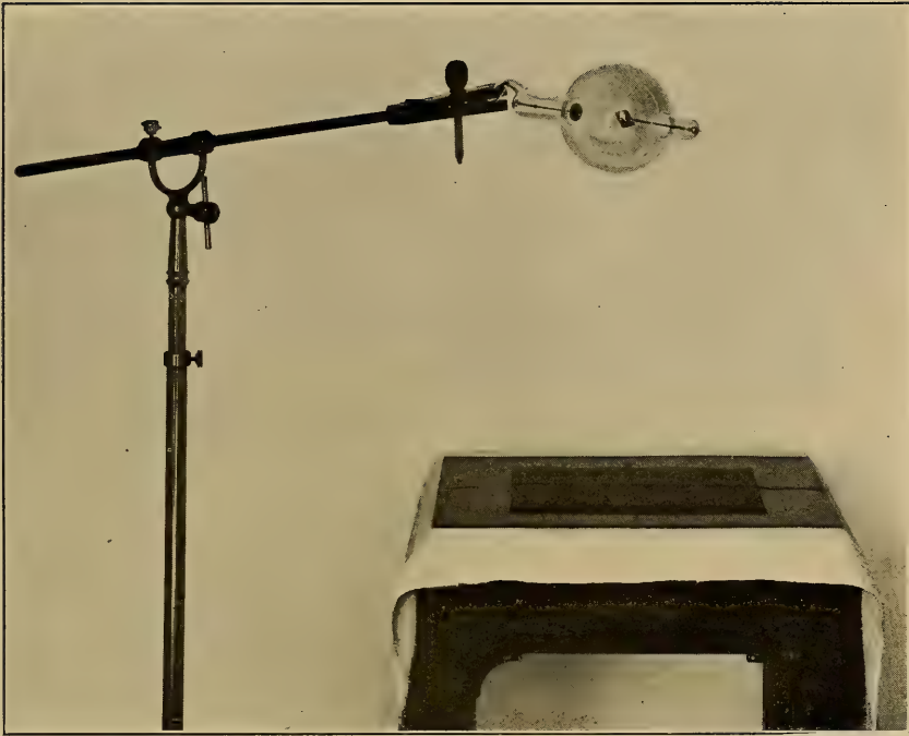
PLATE 35.—Cross-wires for marking quadrants on negative. It is often useful to so mark the negative that it will show the central point of exposure with the field divided into four right-angled parts. This Instruction Plate shows a plate in light-proof envelopes on a base which has two cross wires drawn tightly over at and intersecting in the middle. Focus the tube vertically over the point of intersection and freshly wet the cotton wrapping of the wires with any ink that will mark the skin. Then place the part on the plate and make the exposure. The marks of the wires will be imaged on the negative by the rays and printed on the skin by the ink. Thus the radiograph and part can be compared after the plate is developed and any desired measurements may be made. This device is especially employed in making stereoscopic radiographs. It is well to lay a metallic letter R on the upper corner of the right-hand quadrant to identify it for all examinations.
